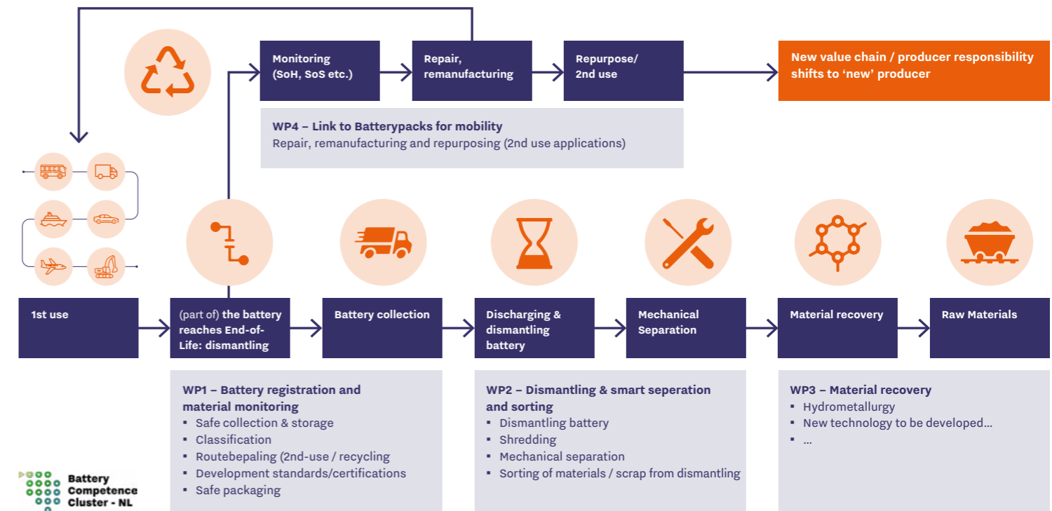
Figure 9: The process for the recycling of e-car batteries
