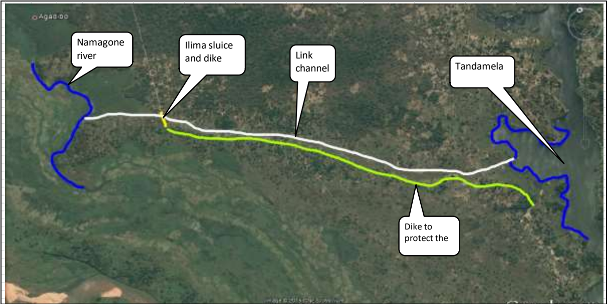
Figure 22 The Future Sluice Complex with Link Channel
