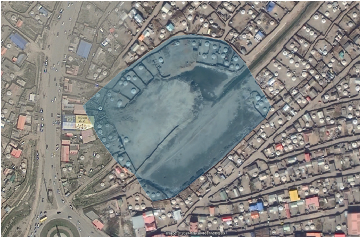
Figure 24: Active area of Nogoon Nuur retention basin in 2005 (highlighted area) and encroachment taking place after 2011.
