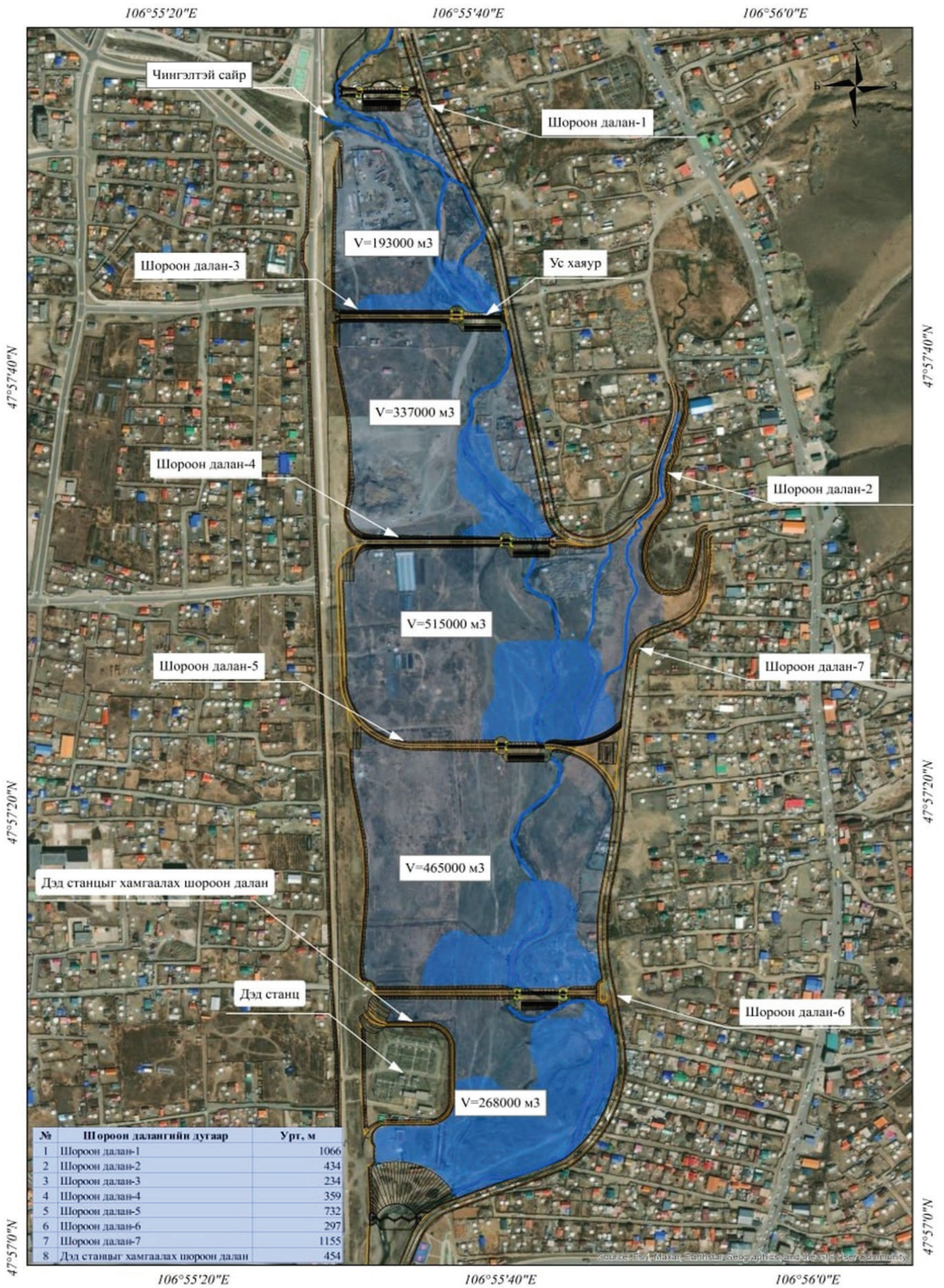
Figure 22: Detailed design of Dambadarjaa retention basins after Selbe revival project (Source: Prestige Engineering, Selbe revival feasibility study report, 2023)
