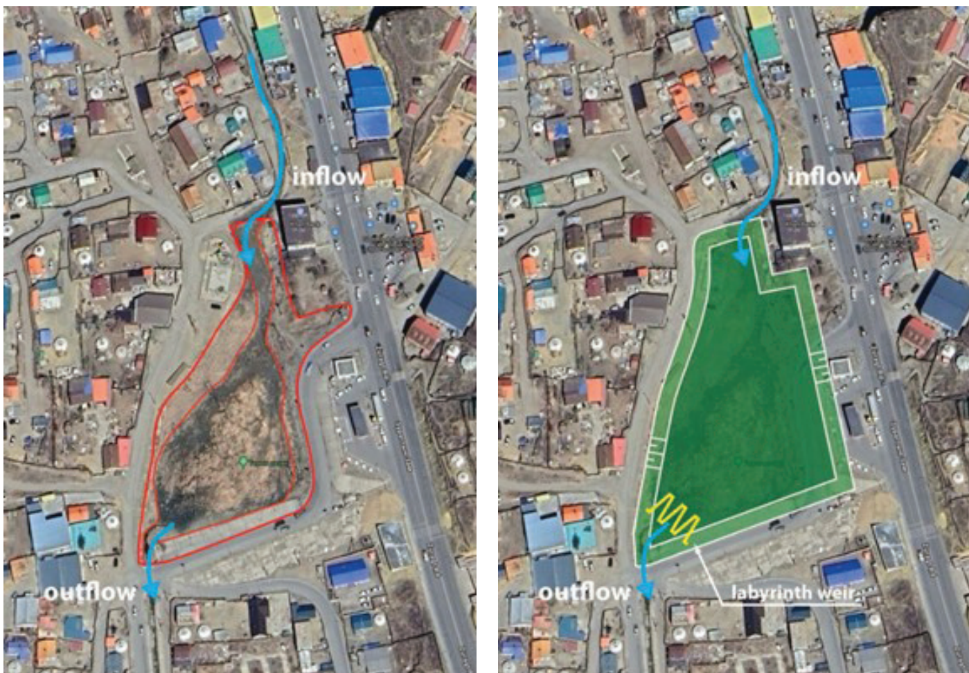
Figure 26: Sambalkhudev retention basin: current condition on left and recommendation on right. (Source: DRRS team)
