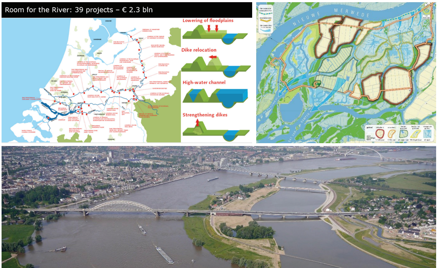
Figure 17: Locations of the 39 "Room for the River" project (left) and an example of the design of the Green River Noordwaard Project (right), Bypass Nijmegen (under).
