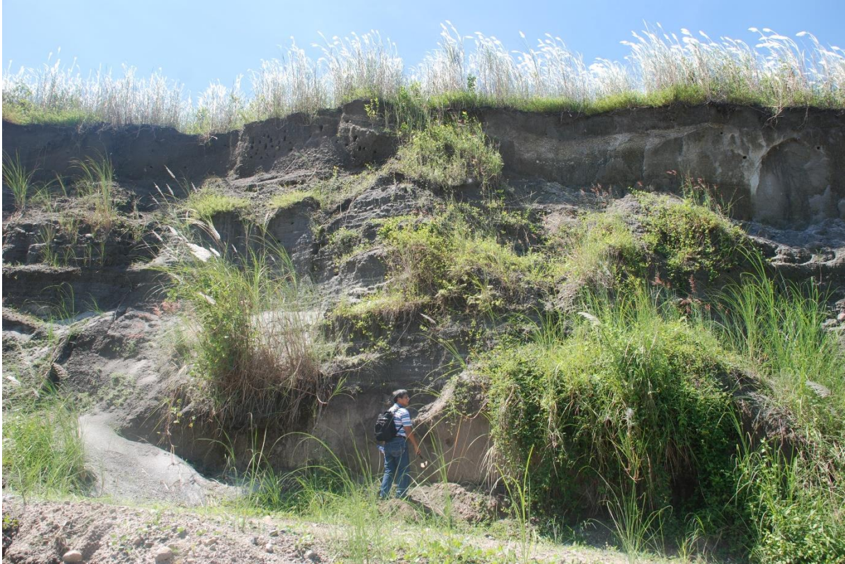
Figure 3.8: DRR team taking a soil sample from the 7m thick ash and lahar deposits near Porac-Gumain River
