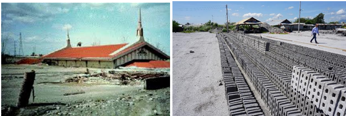
Figure 2.11: Lahar covering human settlements in 1991 is nowadays used as construction material
