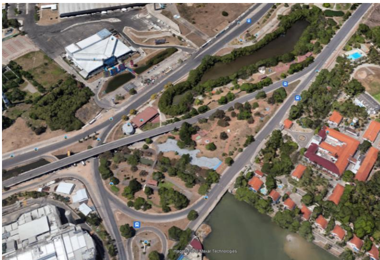
Figure 1: Derby – Tacaruna Canal north with tidal outlet (left) and the possibility to relocate this outlet to the east, allowing to mobilize the capacity of the retention basin shown north.
