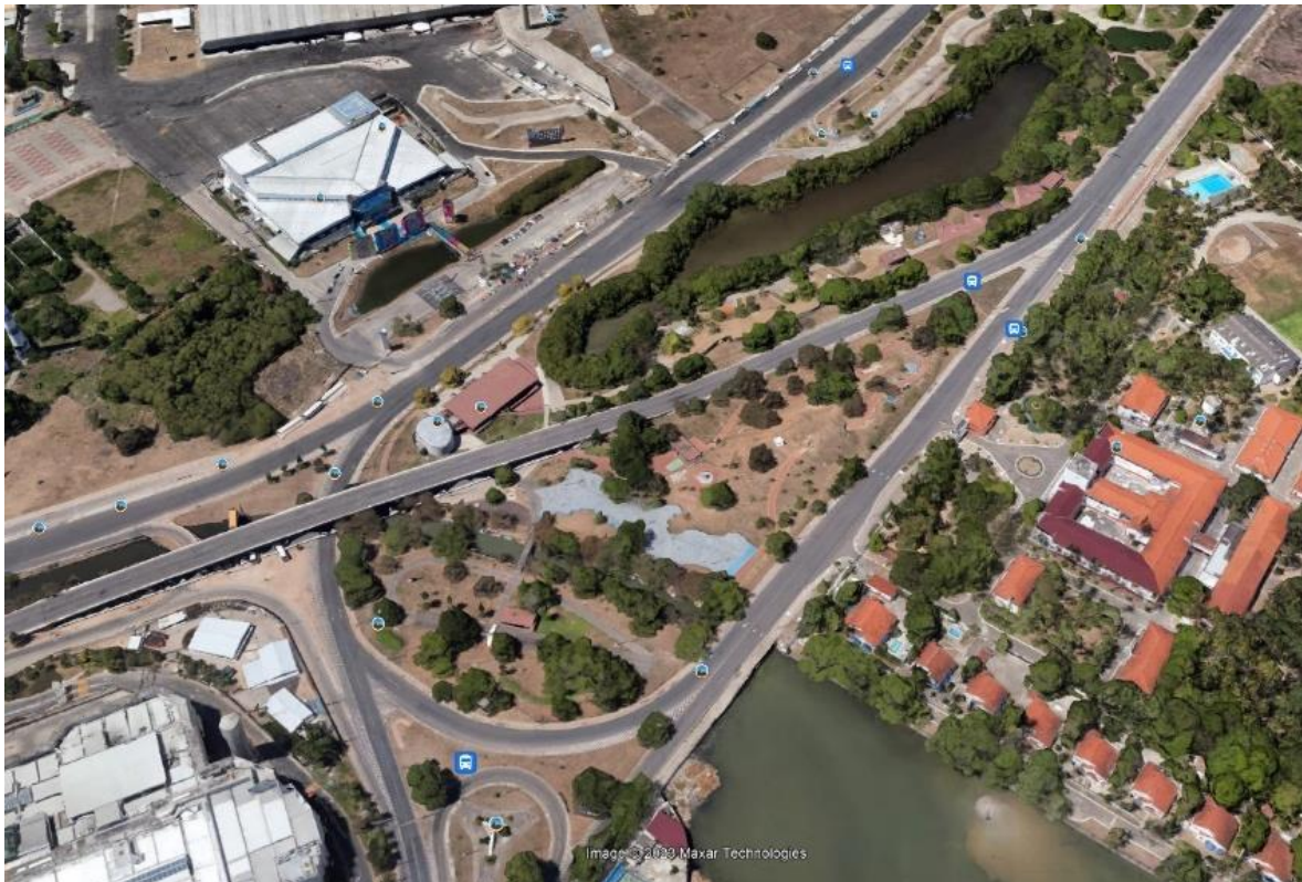
Figure 19: Derby – Tacaruna Canal north with tidal outlet (left) and the possibility to relocate this outlet to the east, allowing to mobilize the capacity of the retention basin shown north or of part of Rio Capibaribe
