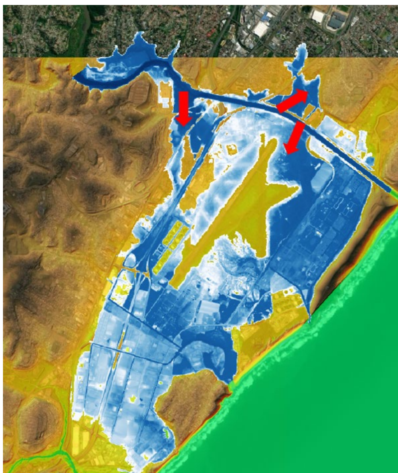
Figure 2-2: Reconstructed April 2022 fluvial event with the three breach locations as red arrows
