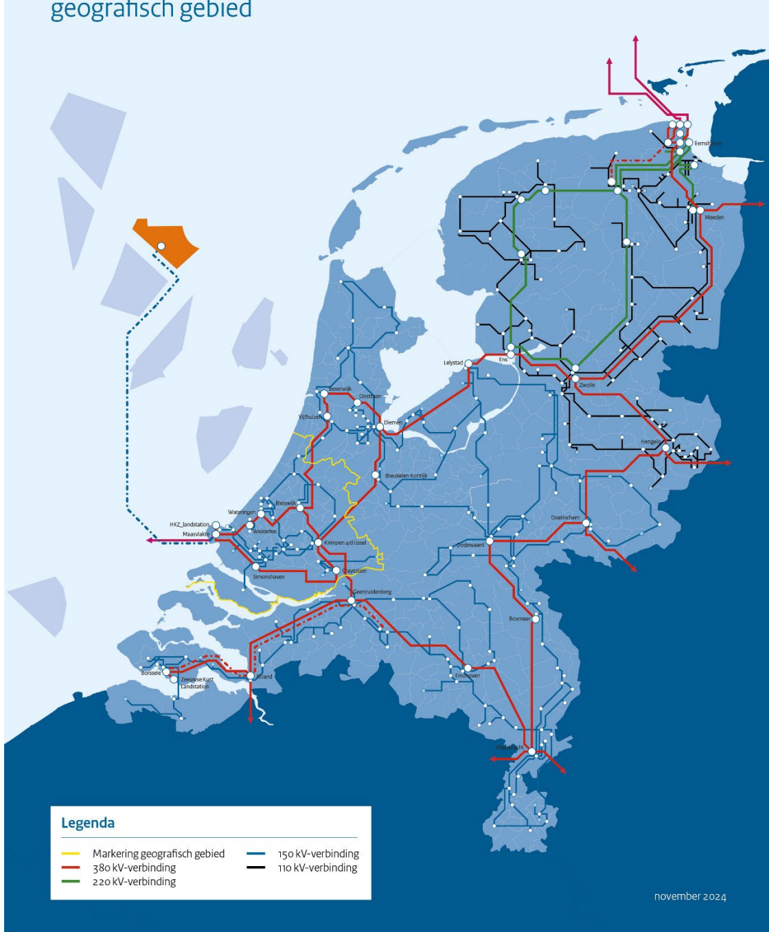
Figure 1. Permit tender IJmuiden Ver Site Gamma-A: marking (yellow line) of the geographical area of the province of South Holland wherein new installations that leads to new electricity demand must be connected to the electricity grid.
